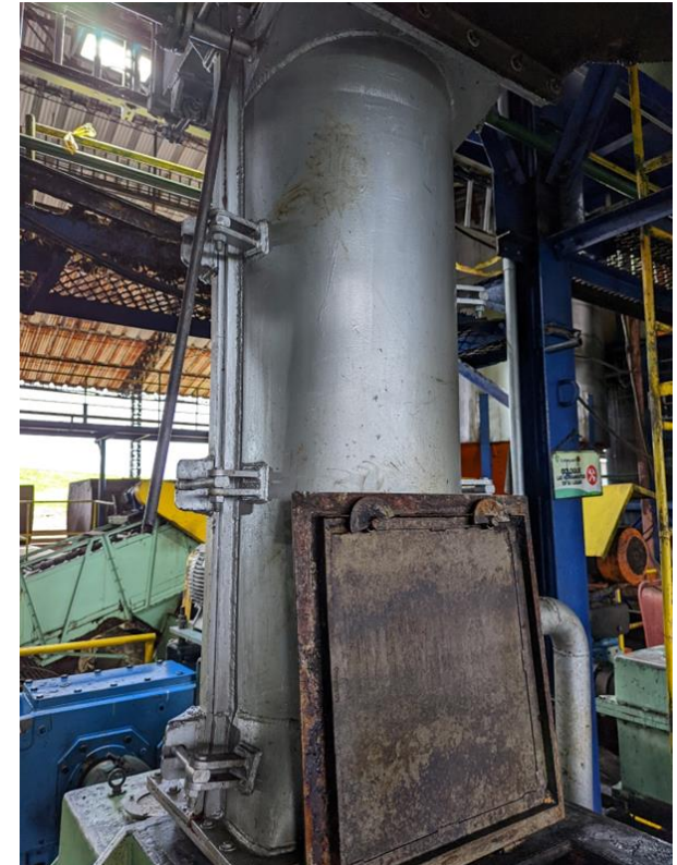
New conditioner unit installed to process kernel-less fruit bunches
