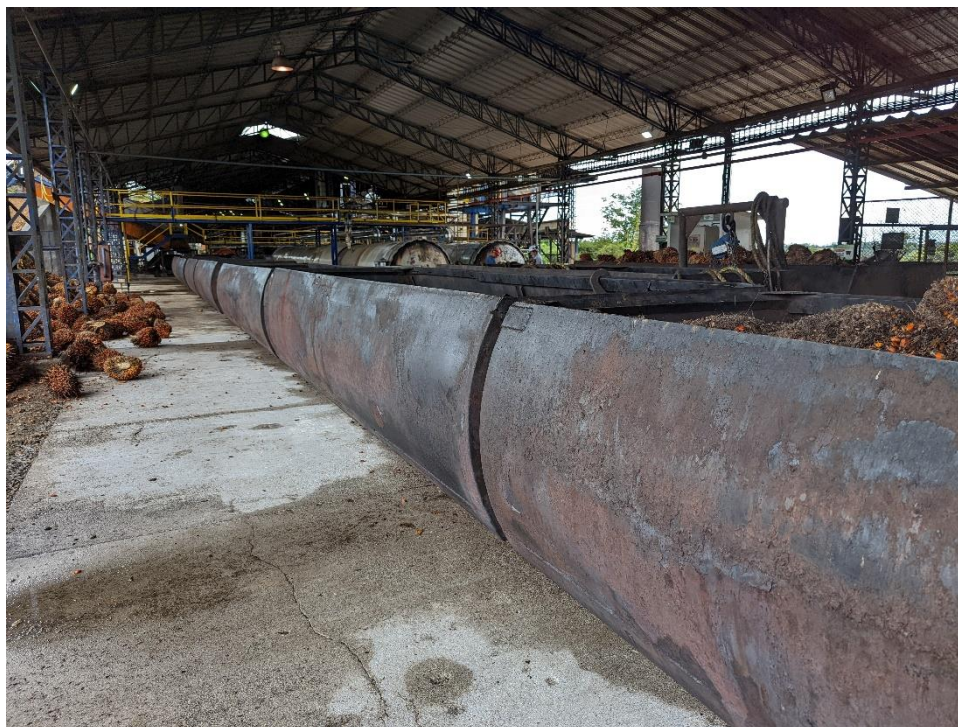
Figure 6 Due to the different oil characteristics, mills need to keep separate milling lines for hybrids and African palm FFB (Hybrid line shown)
